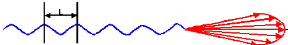
Figure 2.12: The characterization of the undulator radiation. L is the period length of the undulator
